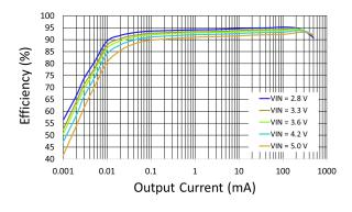
SF30147 is a power management chip featuring ultra-low quiescent current, high-efficiency and high integration, ideal for ultra-low-power wearables and sensor center applications.
